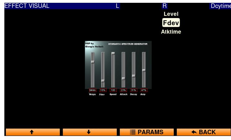
Note that the editing of a parameter of a plugin can also be done through the exclusive use of footswitches, so if necessary, it can be done quickly even during a live performance.
