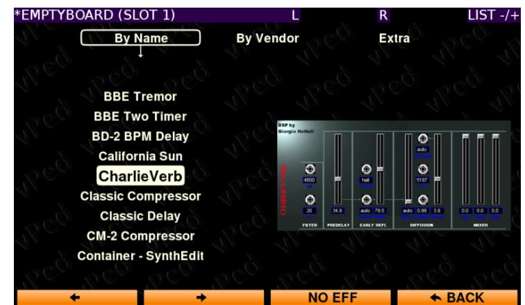
Still in this screen, pressing and holding the "PAGE / ENTER" button for one second, takes you to the screen where you can change the parameters of the plugin you are working on. The methods of intervention are 2:
