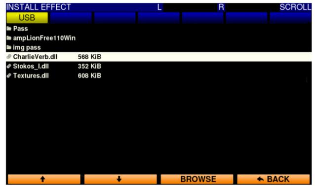
It's possible that some dll installations, require to copy an entire folder (containing for example. Dat file / samples impulses / presets / etc.). In this case, simply drag the entire folder. Exiting the installation page, vPed will install the plugin equally.
