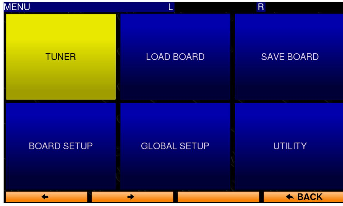
Scroll, with the help of the pedal buttons corresponding arrows on the bottom left, the various panes, and press "PAGE / ENTER" to enter in the corresponding panel. Alternatively, you can use left button of the supplied mouse, or type ENTER on the keyboard (not supplied) if it's connected.
