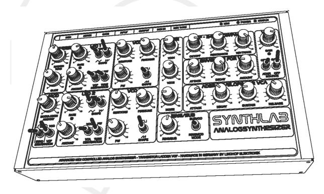
The SYNTHLAB produces sounds 100% analogically as found in traditional analogue synthesisers. The sound production is based upon classical switching systems that originated in the voltage controlled modular systems of the 70's. The low pass filter is put together in the classic "Moog Cascade" tradition which lends the unit similar sound characteristics to Moog synthesisers.
