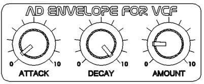
envelope, which is not so important. As we do not possess the hearing to detect slight changes in frequency (as opposed to changes in volume), the VCF envelope curve is therefore in synthesisers generally not as complex as the volume envelope curve. Using the AMOUNT adjustment, the effect of the envelope curve on the filter frequency can be set.
