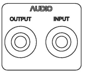
The sockets are 6.3mm jack sockets (mono), making possible a simple integration of the unit with professional studio equipment.
